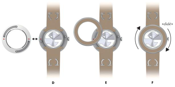
Finally place the bezel aside as shown on the following image D. Match the red dots of the bezel and the case, return the bezel on the case (image E) and screw of a quarter. You must hear a «click» to be sure the bezel is at the right position.
