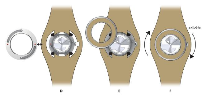
3. Finally place the bezel aside as shown on the following image D. Match the red dots of the bezel and the case, return the bezel on the case (image E) and screw of a quarter. You must hear a «click» to be sure the bezel is at the right position.
