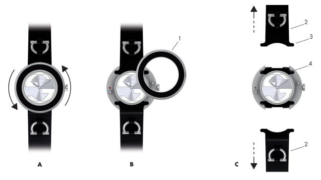
2. Start by inserting the new bracelet and ensure the right position of the inserts.
