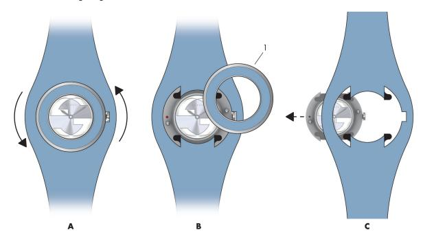
2. Start by inserting the new bracelet in the case and ensure the right position of the inserts.
